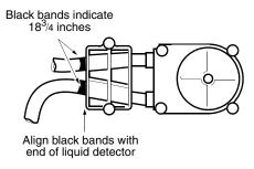
Always maintain 18<sup>1</sup>/2 to 19 inches of tubing inside the pump measured from the edge of the liquid detector block.
